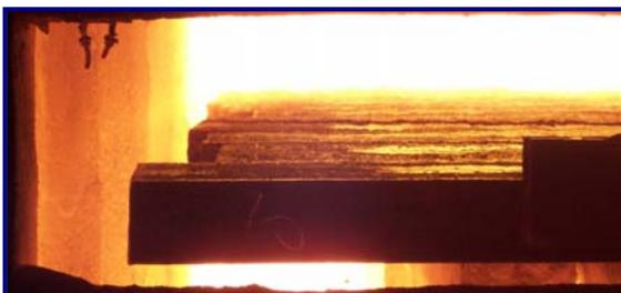
air with massive burners on the side walls of the furnace, both above and below the skids, to heat the slab nearly to its discharge temperature.
