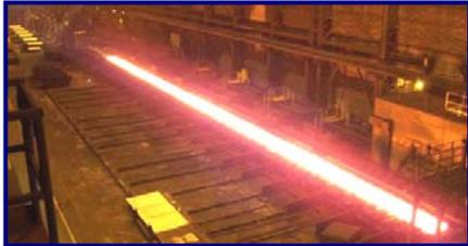
In part because further descaling is not particularly practical once finish rolling begins, the #2 Scale Breaker is the last opportunity to remove oxidation before the finished hot-rolled strip is coiled. Typically, the descaling system in the Hot Strip Mill is very effective at removing primary (from the furnace) and secondary (regrown during roughing rolling) scale.
