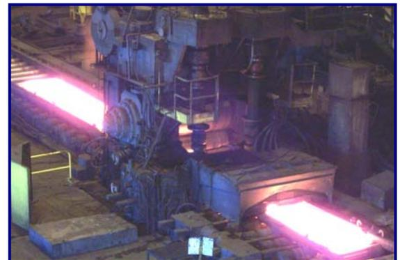
The workhorse roughing mill has 135" wide rolls for rolling 'broadside' (as the first roughing mill is commonly called) to make a slab wider. A 5,000 hp motor drives 42"-diameter work-rolls through 28:1 gears to reduce the slab's thickness by as much as 2-1/2".
