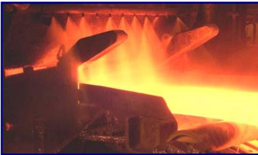
Consequently, a finishing temperature for each product is specified and mill automation will adjust the speed of the first finishing mill stand based on its temperature and the extent to which the bar is expected to cool as it makes its way through each stand, in order to allow the strip exiting the finishing stands to meet the target temperature.
