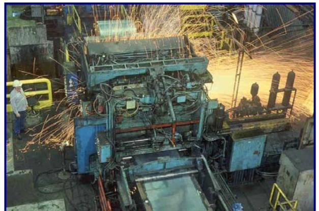
The integrity of the weld is, naturally, very important since strip breaks on the line tend to be time-consuming to repair. For this reason, specific limitations are placed with respect to scheduling orders so as to maintain strong welds between coils of different dimensions and chemistries.
