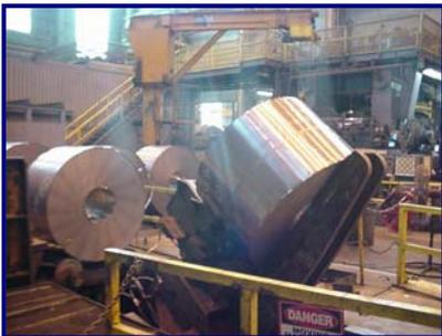
At the exit end, a pair of bridle rolls allow the exit reel to hold the strip under tension while coiling to produce a straight side-wall and prevent the coil from collapsing. Various tension control strategies allow the wind tension to be adjusted as the coil is formed in order to produce a tightly wound coil without contributing to annealing stickers by applying unnecessarily high pressure between the wraps. Coils are upended to an eye-vertical orientation in
