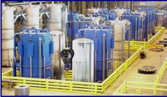
During stress-relief, the first stage reached at around 900 degrees Fahrenheit, the atoms move only small distances, pushed and pulled by surrounding atoms into a configuration in which the internal stresses are reduced but the boundaries between crystals
