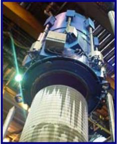
After the step, the burners will fire again to heat the gas stream further to around 1250 degrees. Pre-determined annealing parameters specify a temperature range within which the steel will achieve the desired properties. The cold spot and hot spot requirements are fed into a computer model that uses the thermal transfer properties of the charge to
