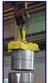
Between coils, spacer disks called convection plates are set to allow the gas stream to circulate along the coil side-walls and between the wraps. Balancing stack stability with heating efficiency considerations in designing the charge, coils and convection plates are alternately stacked up to a maximum height of just over twenty feet. Thermocouples are positioned to monitor the temperatures of the gas stream and base.
