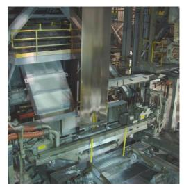
The thickness of the zinc applied to the steel is specified by CSI's customers as a coating weight, in the unit of hundredths of ounces per square foot. An order for 'G-60' seeks 0.60 ounces of zinc on every square foot of steel, which, when evenly distributed, equates to a coating thickness of about one-half of one thousandth of an inch (0.0005") per surface.
