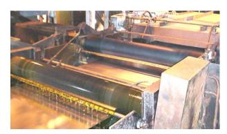
Just before final inspection, the product passes into the stamping area where, when indicated on the schedule, the strip is printed periodically with the product's specifications. The older line uses four 16" diameter ink drums, while the #2 CGL incorporates an ink-jet printer for improved print quality and greater flexibility.
