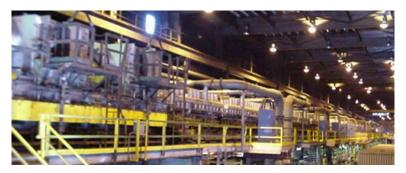
normal operating conditions, the product is annealed for less than a minute. Thin strip at the #2 CGL may spend only 10 seconds in the reducing zones, while heavier gauges at the #1 CGL may take a couple of minutes to reach the necessary temperature. The steel is heated to temperatures typically in the range of 1300° to 1500° Fahrenheit.
