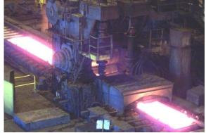
The workhorse roughing mill has 135" wide rolls for rolling 'broadside' (as the first roughing mill is commonly called) to make a slab wider. A
