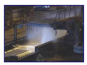
allows physical quality steel grades to retain higher internal stress levels and limits the size of the individual crystals and of the carbides that form within and between the crystals; each of these factors contributes to higher strength levels in the finished hot-rolled strip.
