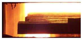
natural gas and preheated combustion air with massive burners on the side walls of the furnace, both above and below the skids, to heat the slab nearly to its discharge temperature.
