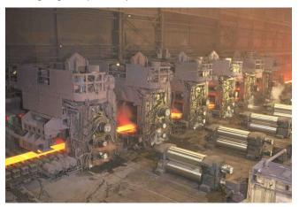
Prior to the finish rolling operation, the head- and tail-ends of the transfer bar will be sheared to square them up, helping to ensure proper threading and tail-out. A final two-stage descaling operation is performed to clean off the scale that has grown on the bar during roughing.
