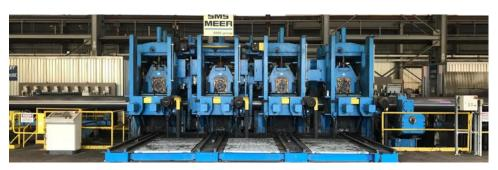
twisting section and four sizing stands consisting of four rolls each. The sizing stands help to make the pipe almost perfectly round, to within a few ten-thousandths of an inch.
