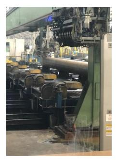
CSITP's #2 Pipe Mill is also equipped for electromagnetic flux-leakage inspection. This inspection is best at detecting surface and subsurface defects, as well as detecting weld-line and other defects. This greatly aids the final inspectors in ensuring that any imperfections that could affect the ability of the pipe to be properly coated are detected and can be repaired.
